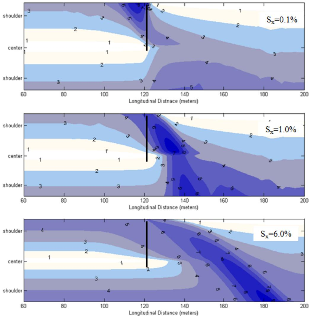
Figure 1 Model of Surface Water Depths (in mm) for various Longitudinal Slopes
