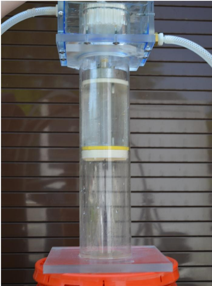
Outer Pipe Column with Cutting Head Inserted.
