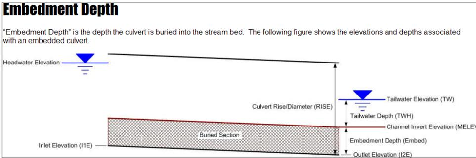
Figure 2. A definition sketch of embedment depth and elevations pertinent to HY-8 computations.
