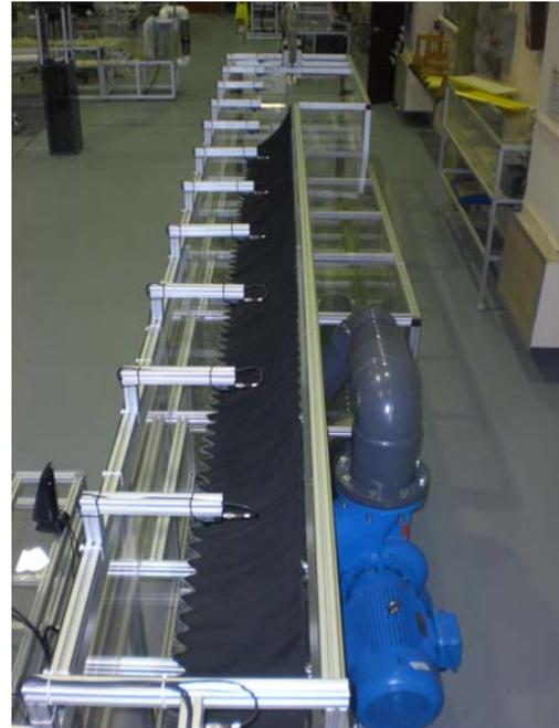
Figure1: Fish Passage Culvert Flume
