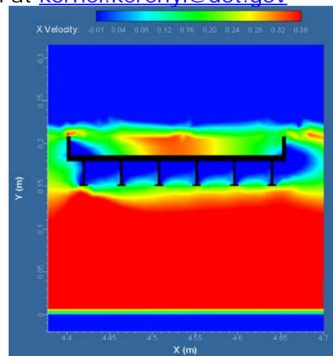
Figure 2: CFD Flow Field Simulation of a submerged bridge deck [index](#)
